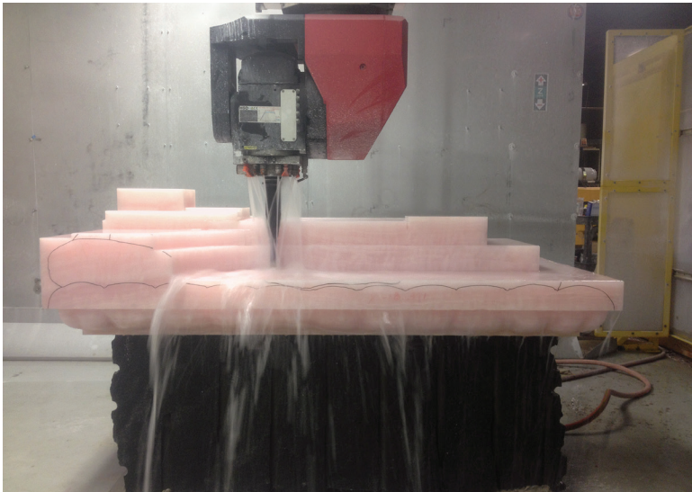
Above and opposite: CNC milling of the stone
