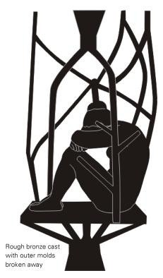
When the bronze is cooled, the outer investment mold is chipped away and the rough bronze is ready for finishing.
